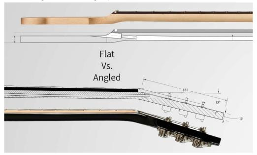
The headstock angle affects the break angle, so if a guitar is too shallow of an angle then the string might slip, but if it is too drastic of an angle for a headstock it may add too much pressure and affect the tuning. Another component to consider is strength. Flat Headstocks are typically stronger because the wood grain direction shifts less with a smaller angle.
