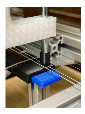
We concluded this was due to excessive friction in the system. We tried oiling the rod so it wouldn't rub up against the structure as much, however achieving equilibrium was still harder than anticipated. In the amount of time we had, we couldn't continue design and testing on the counterbalance system, therefore we can only leave suggestions on what needs to be done. Overall, we solved many of the functional issues and helped make the rig more realistic and effective.
