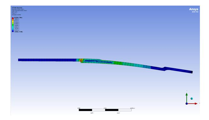
In order to simulate how an *unknown* material will perform under similar tension as a similarly sized neck, we must obtain data from that unknown material to use in our ANSYS model.
