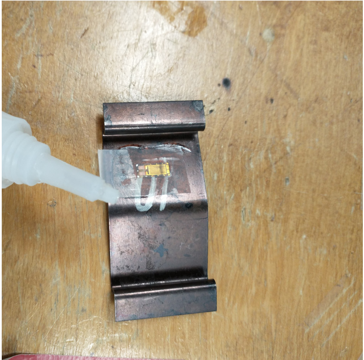
Figure 26: Gluing the strain gage onto the spring
