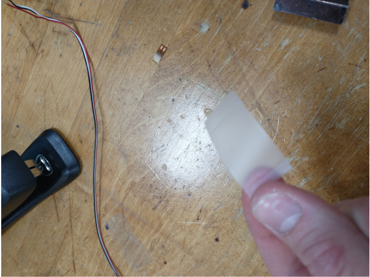
Figure 24: Fold one end of the scotch tape over
