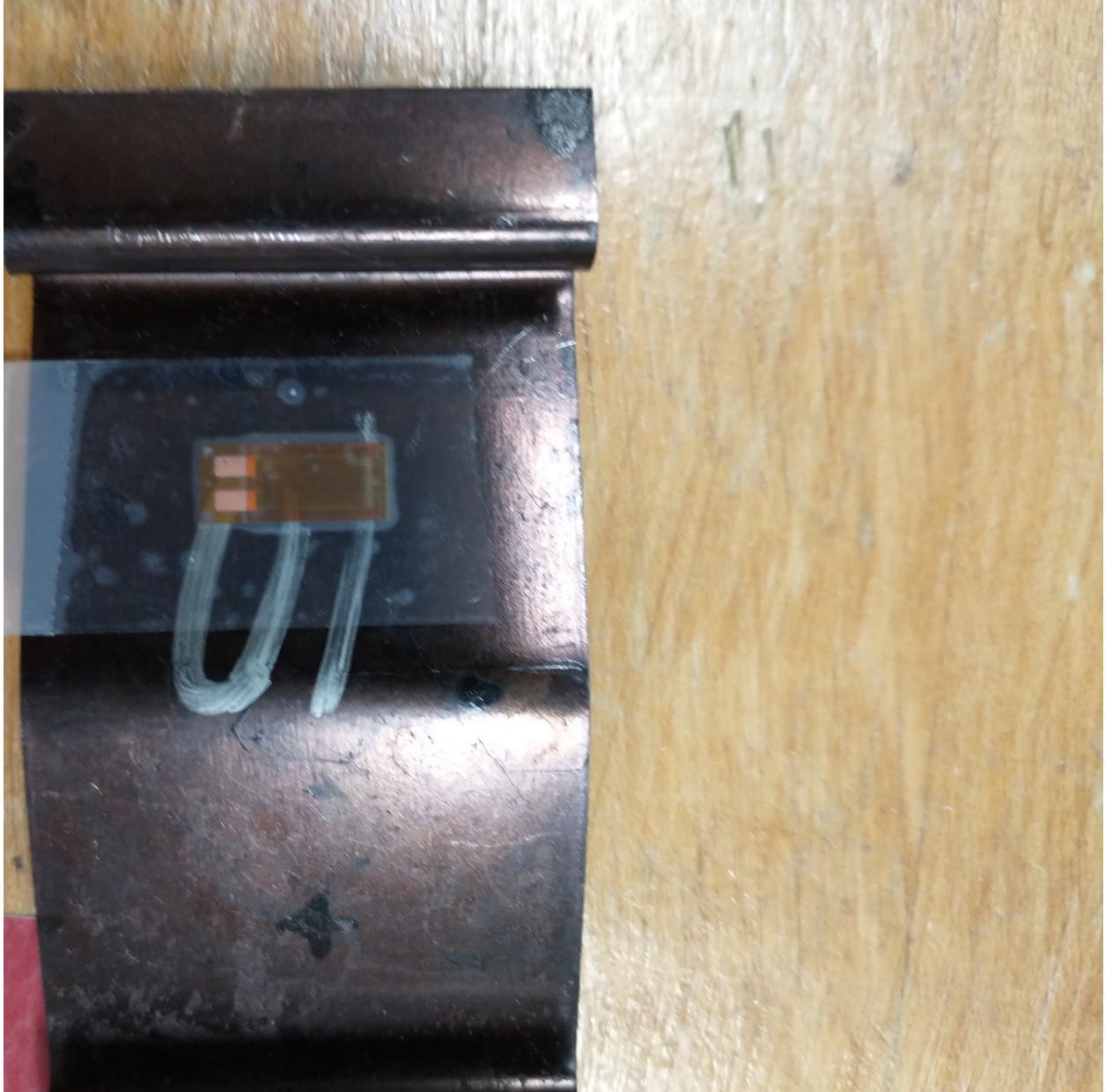
Figure 25: Strain gage attached with tape to the spring
