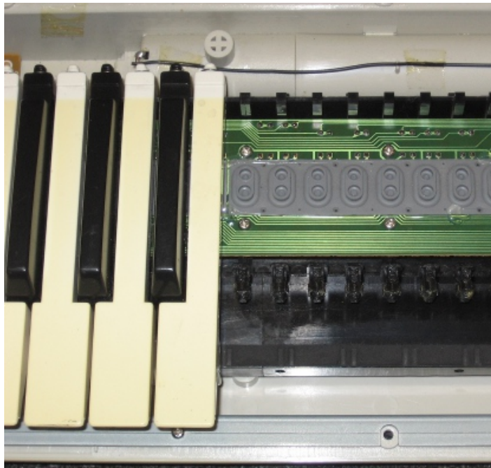
Figure 3. A linear array of pairs of silicone domes in a velocity sensitive keyboard
