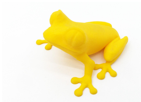
Pict. 25 - the 50-microns treefrog is commonly used as a 3D printing benchmark.
