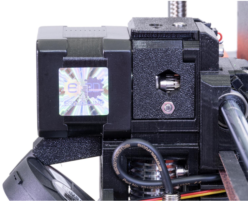
Pict. 40 - Cleaning the extruder - you can see the hobbed pulley through the service hole
