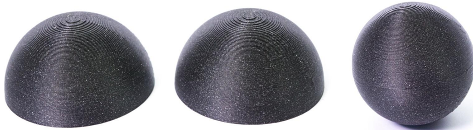
Pict. 29 - A sphere printed in two separate parts glued together
