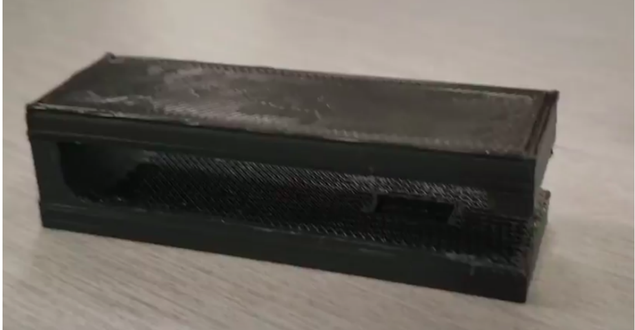
Figure 8: More robust lever button design for limit switches
