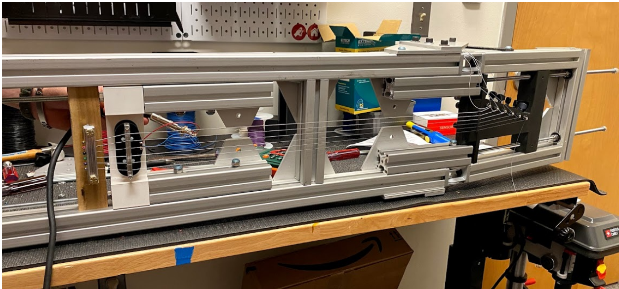
Figure 17: Guitar test rig with the bobbin and new wooden tailpiece module
