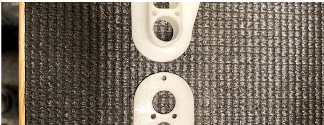
Figure 5: Top and bottom of bobbin machined out of Delrin
