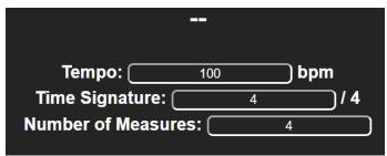
The metronome's default state is '---', and it waits for the user to trigger any of the audio files. When the user triggers any audio files, the metronome turns on and begins counting. For example, at 60 bpm, 4/4, and 4 measures, the metronome count from 1-16, with an interval time of 1 second. After reaching 16, the counter will be set back to 1. This repeats until all buttons are turned off, resetting the metronome to the default state.
