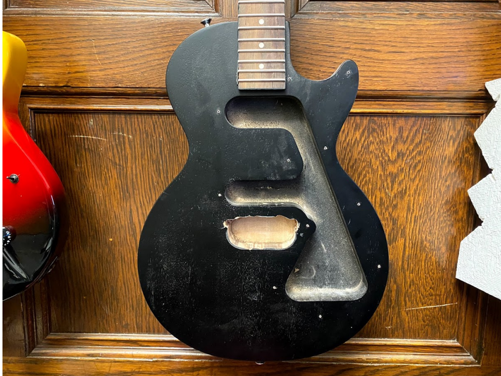
Figure 12: Guitar body with hole routed out to house the pickup
