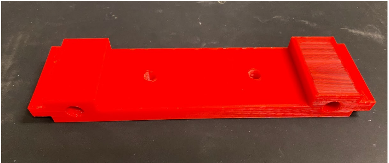
Figure 7: New 3D printed tailpiece (filename: tailpiece_bridge_block_wood)
