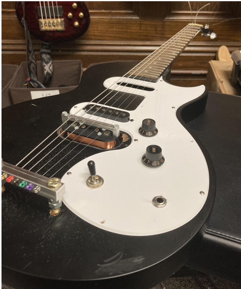
Figure 16: Fully assembled pickup in the guitar
