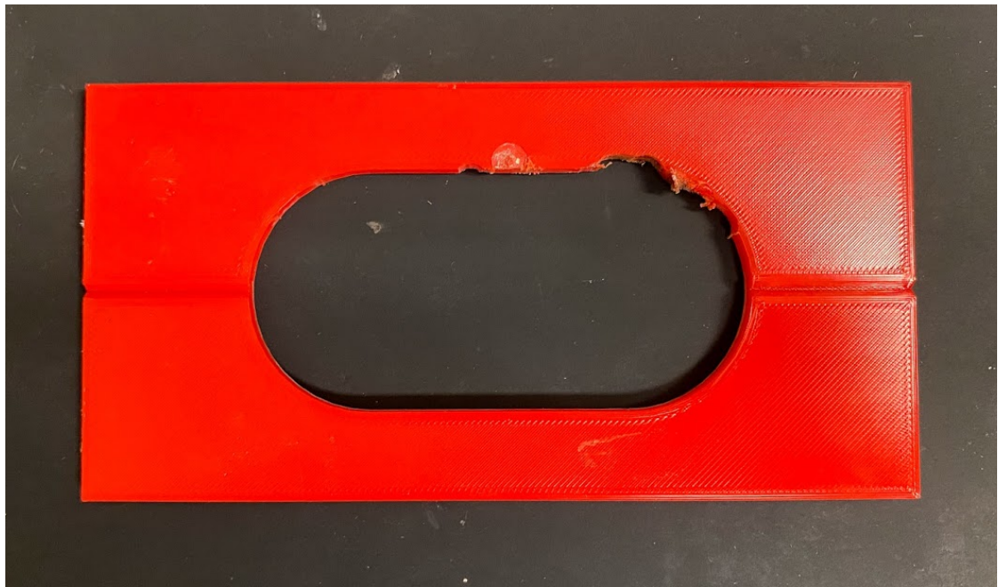
Figure 11: Guide for routing out the hole to house the pickup in the guitar body (file name: Guitar body routing template)
