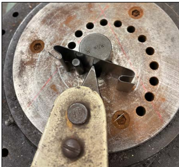
Figure 42: Flat spring with excess piece sheared off in the tube bender
