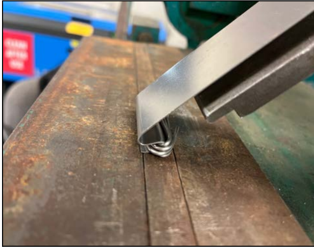
Figure 37: Image of second S bend
