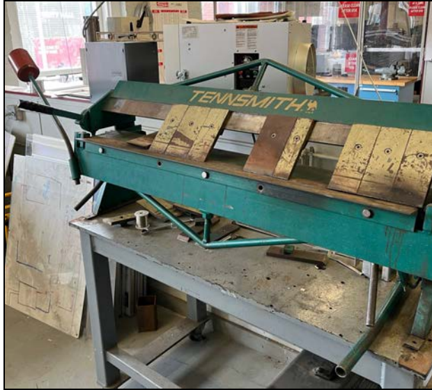
Figure 33: Image of Tennsmith Brake Bender
