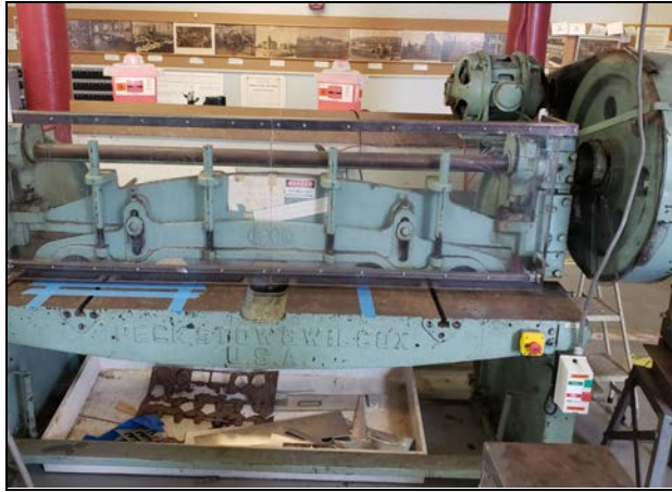
Figure 29: Image of the Peck, Stow & Wilcox hydraulic shearing machine
