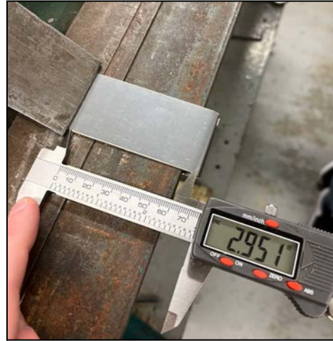
Figure 38: End of spring 2.95in from the brake bender
