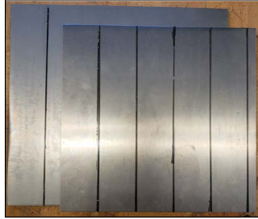
Figure 30: Sheet metal marked to desired width for shearing
