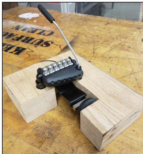
Figure 23: First iteration of rig made of wood
