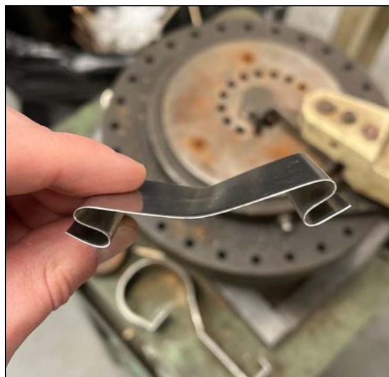
Figure 43: Flat spring with all bends as designed
