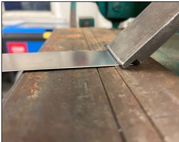
Figure 35: Sheet metal under brake bender
