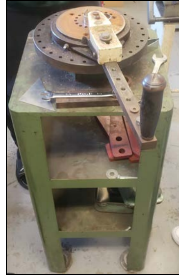
Figure 34: Image of Tube Bender
