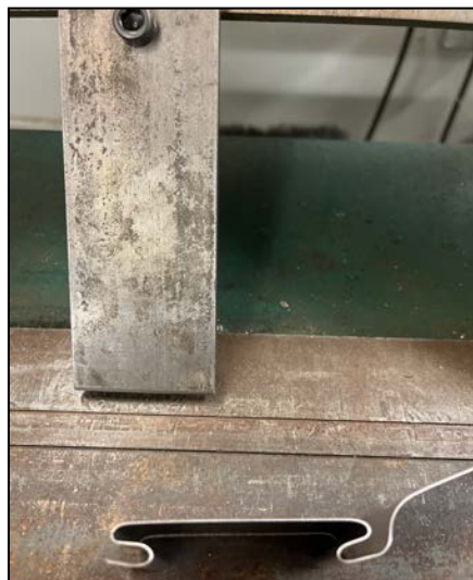
Figure 41: Flat spring with excess material unbent
