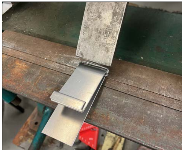
Figure 39: Second S bend with spacer
