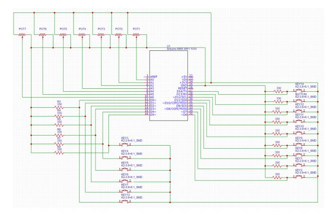
The alternative and more space efficient way would be to use the PCB that was developed to simplify the resistive network. The schematic of the PCB is listed below. The GERBER files for the PCB are also located in the GitLab.
