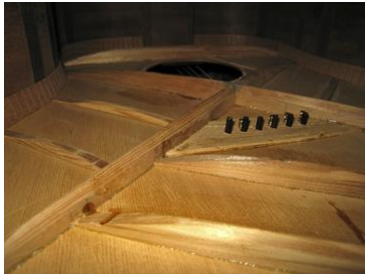
Fig (13) Martin 1945 D-18 with Tapered Bracing
