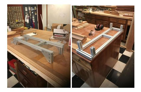
7. The hinge can now be attached to the main assembly and the support bracket and bar attached as well.
