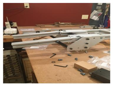
8. Once the hinge is assembled the headstock bar and bridge bar can be attached and the guide rods can be threaded into the desired blocks
