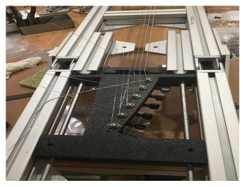
10. Pickup modules can now be place in from the bottom and locked into place as desired or slid into already inserted guide rails
