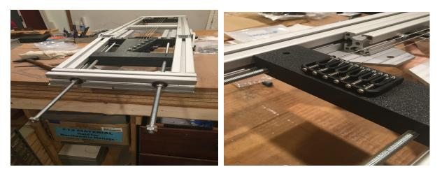
9. Once the blocks are in place and locked in with rods the nut module can be put in place and the system strung
