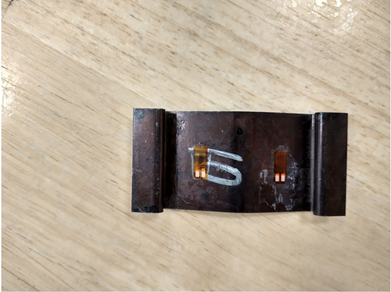
Figure 27: Both strain gages glued to the spring
